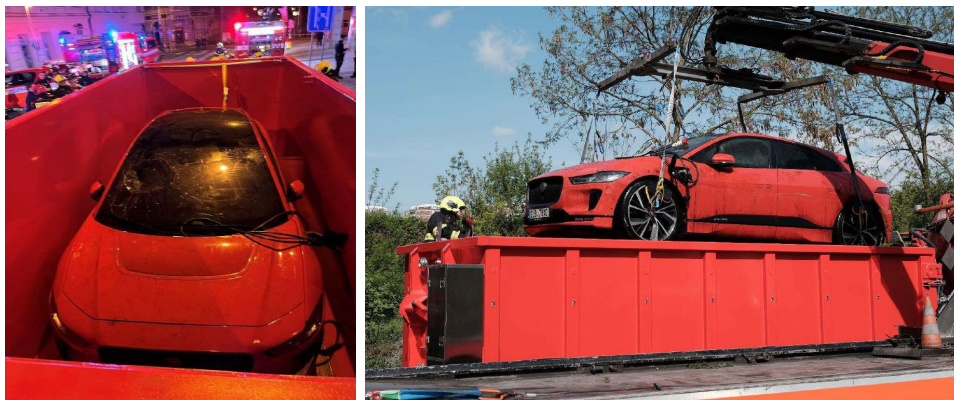
FIGURE 14 (LEFT) EV PLACED INTO IMMERSION CONTAINER 91 ; AND, (RIGHT) EV BEING REMOVED FROM IMMERSION CONTAINER 91 .
