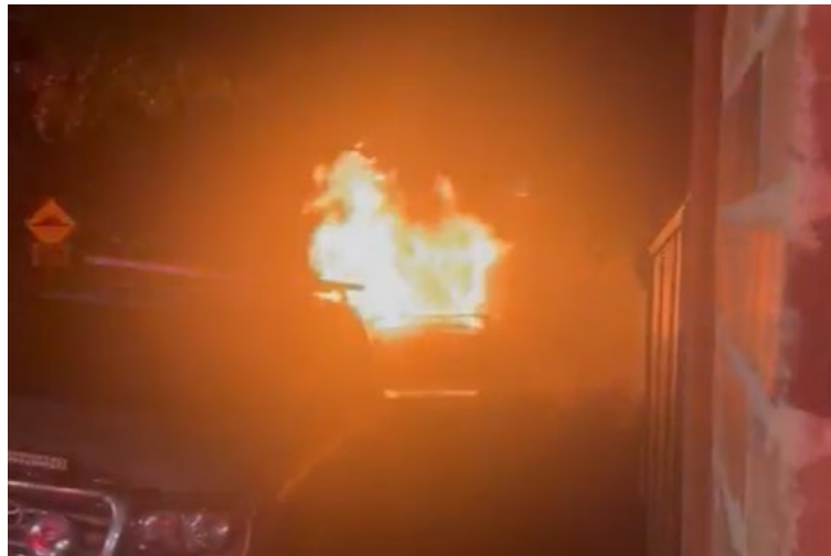
FIGURE 11 IMAGE FROM FOOTAGE CAPTURED AT THE SCENE IN CAMPERDOWN WHEN THE DOOR OF THE PHEV WAS OPENED AND FLAMES ERUPTED FROM THE VEHICLE CABIN.
