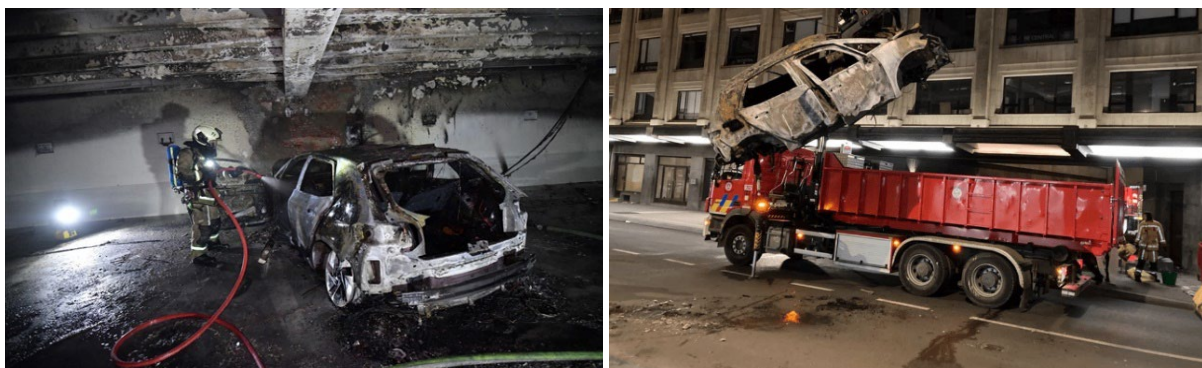
FIGURE 12 (LEFT) BURNT OUT EV IN THE RAVENSTEIN STREET PARKING GARAGE IN BRUSSELS, AND (RIGHT) EV REMAINS BEING LIFTED INTO A CONTAINER TRUCK FOR IMMERSION (THE BRUSSEL TIMES, 15 FEBRUARY 2022 89 ).
