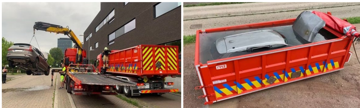
FIGURE 4 AN EV BEING CRANED INTO A CONTAINER (LEFT) AND IMMERSSED IN WATER (RIGHT) IN LEUVEN, BELGIUM FOLLOWING A THERMAL RUNAWAY INCIDENT (SOURCE: OOST VLAAMS BRABANT 2021 59 )
