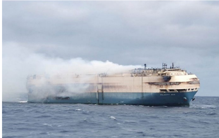
FIGURE 2 A FIRE BROKE OUT ON THE FELICITY ACE ON 16 FEBRUARY 2022 IN THE NORTH ATLANTIC OFF THE COAST OF PORTUGAL (SOURCE: REUTERS 2022 20 ). THE SHIP WAS CARRYING 3965 NEW VEHICLES FROM GERMANY TO THE USA. THE ORIGIN OF THE FIRE HAS REPORTEDLY BEEN ATTRIBUTED TO THE LIB FROM A PORSCHE 23 .
