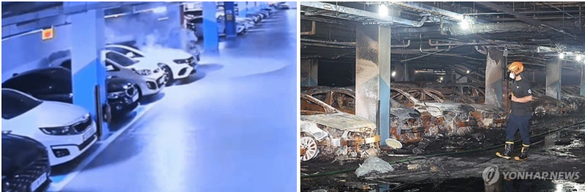
FIGURE 17 (LEFT) IMAGE FROM CCTV FOOTAGE SHOWING THE VEHICLE OF ORIGIN RELEASING PALE VAPOURS AS IT ENTERED THERMAL RUNAWAY, BEFORE FLAMES ERUPTED (SOURCE: KOREA JOONGANG DAILY 2024 19 ) 19 . THE VEHICLE WAS NOT ON CHARGE AT THE TIME AND THE OWNER REPORTED THAT THE VEHICLE HAD BEEN PARKED FOR THREE DAYS BEFORE THE FIRE WITHOUT ANY APPARENT ISSUES 97 . (RIGHT) AFTERMATH OF THE INCHEON APARTMENT CARPARK FIRE ON 1 ST AUGUST 2024 (SOURCE: YONHAP NEWS 2024 96 )
